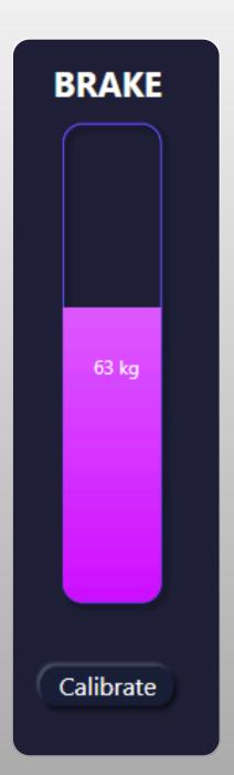
For the Mercedes AMG GT3, the maximum braking force is set at 63 kgf (≈ 618 N), equivalent to a hydraulic pressure of about 112 bar with a 17.8 mm master cylinder and a 5:1 pedal ratio. This value serves as the reference for pedal calibration.
