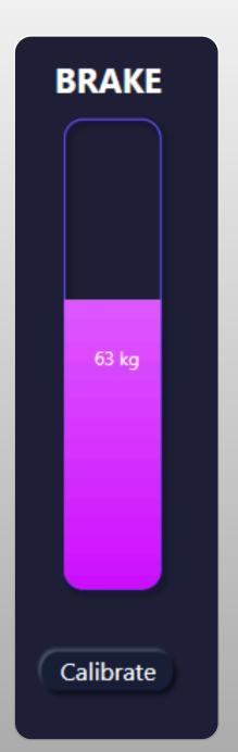
For the Mercedes AMG GT3, the maximum braking force is set at 63 kgf (≈ 618 N), equivalent to a hydraulic pressure of about 112 bar with a 17.8 mm master cylinder and a 5:1 pedal ratio. This value serves as the reference for pedal calibration.
